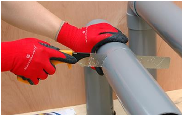
A picture of the pipe blade (well actually a different, hook-fitting, blade but with the same tooth pattern) in use.
