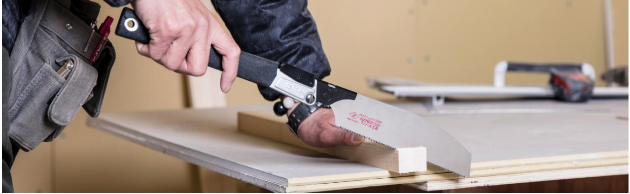
The H-200 Handy utility blade, with folding V handle, cross-cutting timber.
