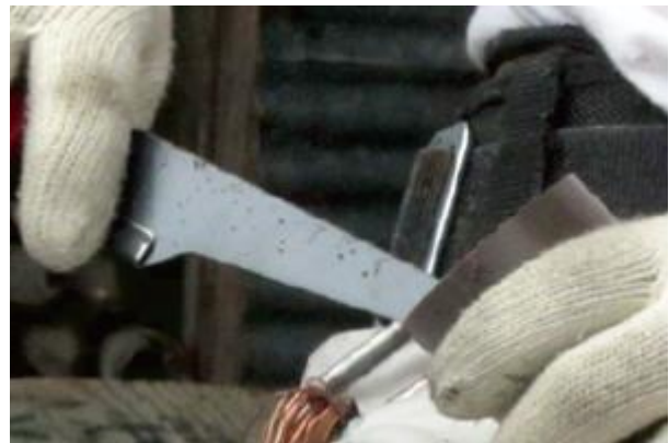
Using the back of the H-180 Waistern metal blade for deburring.
