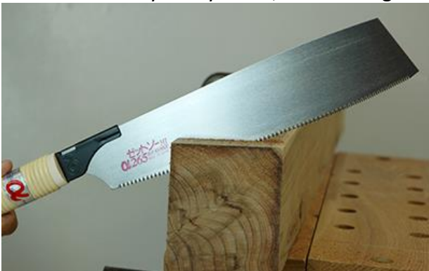
The H-200 Handy utility blade, with folding V handle, cross-cutting timber.
