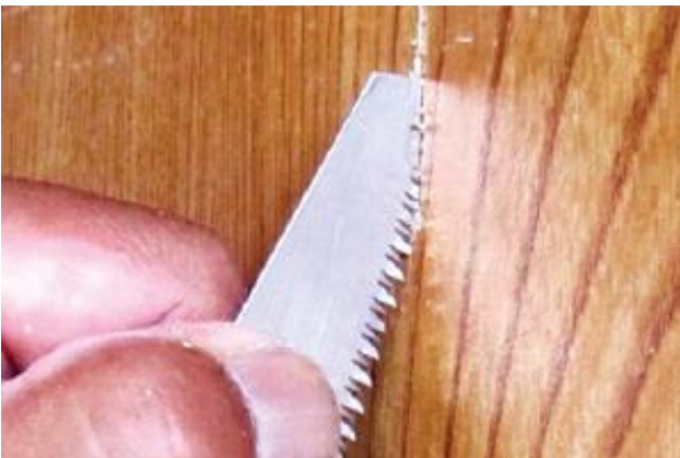
Using the H-180 Waistern woodworking blade to start a cut in the centre of a panel.
